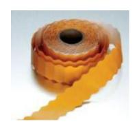
True Indicating Radiation Chemical Process Indicator labels contain no lead or other toxic heavy metals. The Indicators are manufactured to monitor whether radiation conditions were met at the point of application, using latex-free pressure sensitive adhesive. The indicators are designed for use with radiation operating as low a 10 kGy, with optimal color transition at dose levels of 25 kGy.
