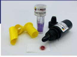
**SCBI Activation (Optional):** Depress the cap in a downward motion until an audible clip is heard and the glass media ampule contained within is crushed. Ensure that the disc is immersed in the growth medium. Activate one SCBI which has not been exposed in a sterilization process as a Positive Control.
